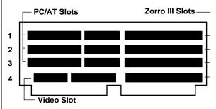
of XT or AT- style boards. The remaining Zorro III slots support both 24 & 32-bit Zorro boards.
