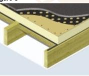
Staggered board joints over roof joists
