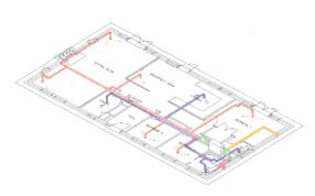
Ducting connects the stale air exhaust grille to the Heat Recovery unit and extracts via ducting to all the wet areas of the property. The stale air passes through the cross-flow heat exchanger and typically 65-70% of the heat normally lost via trickle vents is recovered.
