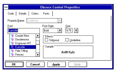
Each page contains an OK button which, if pushed causes the current contents of all the pages to be used in re-creating the barcode image. The pages also contain a Cancel button which may be used to close the Property pages dialog and discard any changes made.
