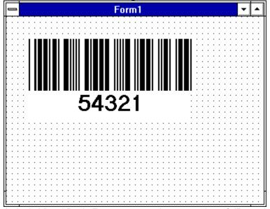
A single Visual Basic Form may contain any number of dBarcode controls. The first to be added will be called Dbcocx1, the second Dbcocx2, and so on; the names may be changed by the user by modifying the Name property within the Visual Basic Properties box.
