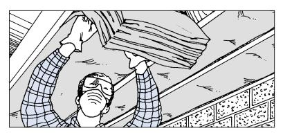
Press the insulation between the floor joists above your head starting at one end and working out until the cavity is filled. Insulation with a vapor retarder should be used, with the vapor retarder facing up towards the heated area of the home. The insulation should be installed up against the subfloor. The insulation will stay temporarily in place.
