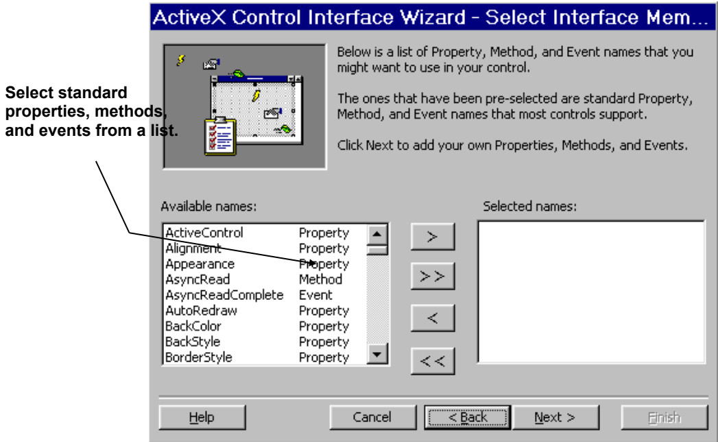
Figure 14. The ActiveX Control Interface Wizard gives developers a list of properties, methods, and events for common controls.
