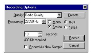
**Quality**: The quality list allows you to quickly select the format of your sample from a list. The items on the list can be added to by pressing the <u>presets</u> button, which lets you define new sample qualities.
