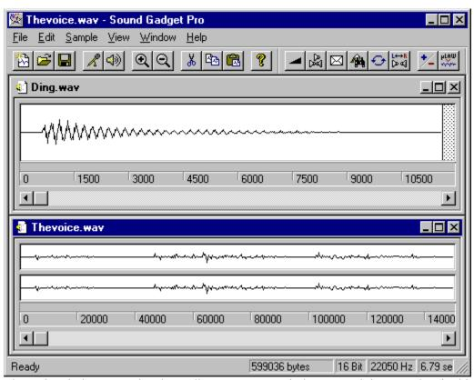
The main windows contains the <u>toolbars</u>, two MDI windows containing samples (in this, the example, the top window is a mono sample and the bottom is a stereo sample), and any currently active toolbars.
