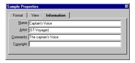
The information sheet sets extra information about the sample that will be saved if the sample is saved in .WAV format. It is useful if you want to keep a record of the source of a particular sample.
