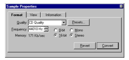
The format sheet allows you to set the current metrics for the sample. Any changes made are not permanent, and can be reversed by pressing the Revert button. If you want to change the format of the sample to the new metrics, then press the Convert button, which performs the same function as the <u>Convert dialog</u>. Sample presets also work in the same way.
