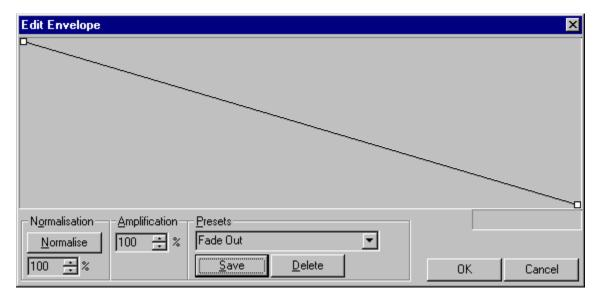
The sample envelope dialog changes a sample's volume with respect to time. Manipulate the handles in the top window to create a path for the envelope to follow.
