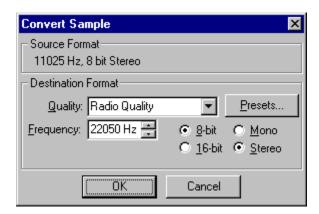
Convert will change the current sample to the destination format. Alter the format manually, or use any of the quality presets, which you can change with the <u>Presets</u> button.
