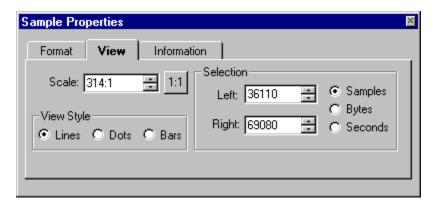
The view sheet changes the properties of the view of the sample. You can change the scale (number of samples / pixel), the style (how the sample is drawn), and change the position of the cursor or change the parameters of the current selection.
