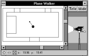
The **Plane Walker Window** shows a <u>Floor Plan</u> of the **3D Space** and includes <u>Pinocchio</u>, which you can use to move the **Camera** around the 3D Space. The Plane Walker Window also includes the <u>Camera lcon</u>, which you can use to adjust the **Height, Angle (Tilt)** and **Zoom Qualities** of the Camera.
