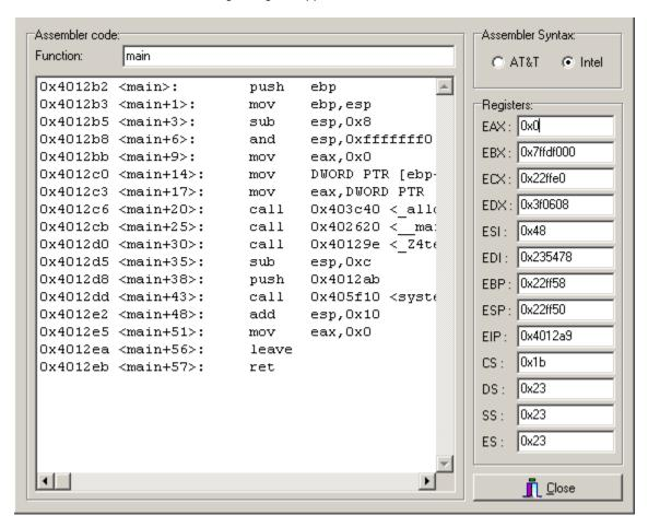
On the left, you can find the assembler instructions of the current function. You can display the assembler code of any other function by typing its name in the *Function* field, then pressing the Enter key. You can also select the syntax of the assembler instructions: AT&T or Intel.
