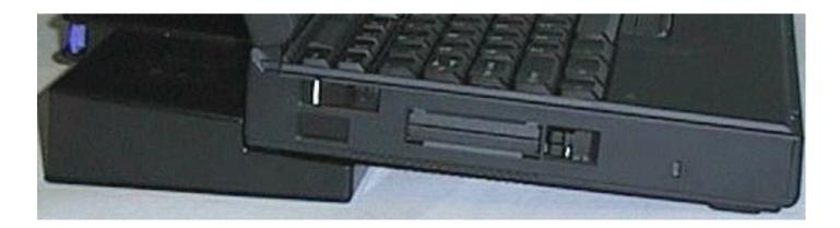
ThinkPad 380 held at ergonomic tilt when connected to port replicator
