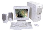
standard P-III system with 64 MB of RAM, this machine has a 440ZX Intel chipset motherboard, which provides three PCI slots and one shared PCI/ISA slot for expansion. Two USB ports are also provided. The cabinet is quite spacious and has ample space for installation of extra drives. An SiS AGP card with 4 MB video memory and a 14-inch Viewsonic monitor are responsible for graphics.
