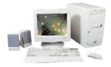
ased on the new Intel 810 chipset, this computer integrates features like 3D graphics and audio directly on the motherboard. Running a speedy Celeron 433 MHz with 64 MB SDRAM and a 6.4 GB Seagate U4 hard
