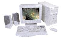
his system with a Celeron 400 MHz processor and 64 MB of RAM uses a 440LX Intel chipset motherboard with an integrated Creative PCI 128 sound chip. Three PCI slots and one ISA slot provide ample
