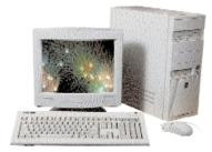
esigned for basic office applications, this P-II 350 machine has only 32 MB RAM and does not feature a soundcard or speakers as standard components. The PC s Intel SE440BX2 motherboard has three PCI
