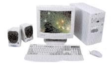
his P-III 450 MHz-based system has 64 MB of RAM on an Intel 440ZX motherboard, which also houses three PCI slots, one ISA slot and one shared PCI/ISA slot. The cabinet used is an ordinary looking
