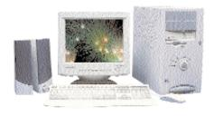
his P-III 450-based system has an ample 128-MB of RAM providing very good performance. The system uses a 440ZX Intel chipset mother-board with two PCI slots, one ISA slot and one shared PCI/ISA slot. The
