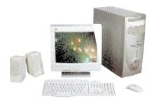
he system features a P-III 450 processor with 64 MB of RAM. An Intel SR440BX motherboard with an integrated nVidia Riva TNT graphics chip having 16 MB memory and an inte-
