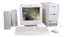
ne of the most feature-rich machines in this roundup, the Aptiva 240 integrates an impressive set of components and peripherals. Based on a K6-2 350 MHz processor with 64 MB SDRAM, this reasonably fast machine
