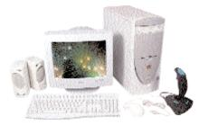
he system features a P-III 450 MHz processor and 64 MB RAM installed on an Xoel 2000 chipset-based allin-one motherboard. The motherboard has an onboard SiS 620 graphics with 8 MB of shared video memory, Sound Pro
