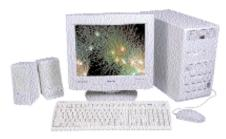
his average-looking P-III 450 system comes with a 15-inch Samsung 55E monitor and a Trident 4 MB AGP card with TV-out ports that provide reasonable graphics; the RAM though is a mere 32 MB. The 440ZX Intel chipset
