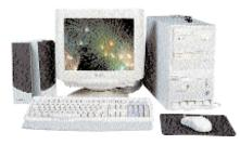
his high-end system is based upon a P-III 450 with 64 MB of RAM and a speedy 4.3 GB Quantum Fireball CR hard disk that features an ATA66 interface. However, the motherboard houses a 440BX-based chipset
