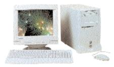
ased on a Celeron 400 and an SiS 5595 chipset, this computer integrates the graphics adapter directly on the motherboard. The graphics card consists of an SiS 540 onboard graphics card that shares main memory and uses it as video RAM. There are
