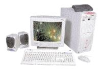
imiting the overall performance of this P-III 450 MHz-based system is the 32 MB RAM, which is no match for the P-III 450 processor. The i440BX motherboard supports both Slot
