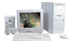
his high-end system incorporates some of the best hardware available for an entertainment and game machine. An AOpen mother-board with a P-III 450, 64 MB of SDRAM, an S3 Savage 3D accelerator
