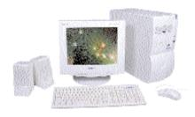
system with average components, the machine features a P-III 450 processor and 64 MB RAM installed on a 440ZX Intel chipset motherboard. Two PCI slots, one ISA slot and one shared PCI/ISA slot provide room
