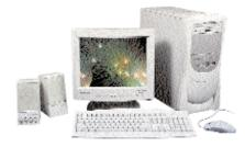
his budget computer is based on a 440ZX chipset and is a good alternative to more expensive BX-based systems. Running on a Celeron 400 MHz with 32 MB of 100 MHz SDRAM, this machine is suited to home and low-power
