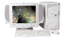
his good-looking P-II 400-based system features only 32 MB of RAM. The base of the system is a 440ZX Intel chipset motherboard with two PCI slots and one slot each of ISA and shared PCI/ISA slot. The ATX cabi-
