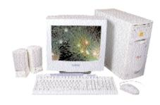
his P-II 350 based system has only 32 MB of RAM installed on a 440ZX Intel chipset motherboard that houses two PCI slots, one ISA and one shared PCI/ISA slot. A 15-inch Box mon-
