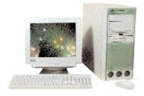
esigned for the office user, this PC sports a tower casing that does not have any screws on the slot interfaces, enabling you to add new components effortlessly.
