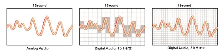
The effect of increasing sampling rate and number of bits on the purity of the output (digital) signal. The higher the sampling rate and the number of bits used, the closer is the approximation of the output digital signal with the input analog signal.
