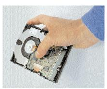
While holding a hard disk, the electronic underside should not be touched
