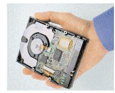
Always hold a hard disk by the edges to prevent damage due to static discharge
