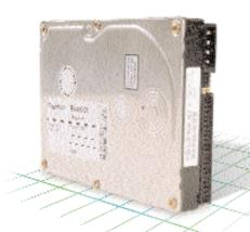
This 3.5-inch IDE hard disk is part of Quantum's new Ultra ATA/66 or UDMA mode 4 range of hard disks. Though rather plain-looking, this hard disk has a formatted capacity of 8.4 GB and two platters that give it a total of four recording surfaces.
