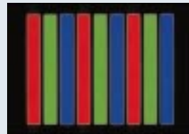
Image 3: In the Aperture Grille CRT tube, the primary colour stripes flow vertically over the entire length of the screen.
