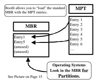
To get other partitions to show up in the operating system, as you can see from the figure above, you must assign the partitions to be loaded (up to four). Failure to correctly load the **MBR Details** section of the Boot Item—see the screen capture in Set up the Normal Boot Menu on page 15—is the most common cause of missing partitions.
