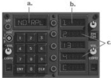
Figure 7 - Up Front Control Panel
