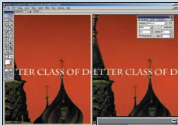
What jpeg does to text. Notice the halo effect at the dome edges
