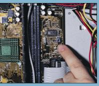
**1 O**<sup>our</sup> old PII 350MHz used an FSB setting of 100MHz, but our new 933MHz PIII requires a setting of 133MHz. Most older motherboards change their FSB using jumpers identified in the manual, and on the P2B these are labelled FSO to FS3. These should all be set to 1-2 to drive the FSB at 133MHz and the PCI bus at the correct 33MHz setting. Note that we will now need to use like the PIII 800E. This will, however, need PC133 memory.
