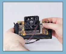
All CPUs need heatsinks and fans to keep them cool, so we bought a good one from www.overclockers.co.uk - any decent heatsink for an FC-PGA processo should do the trick. For best results, first spread a very thin layer of thermal paste on top of the small metal square in the middle of the plastic CPU frame overclockers.co.uk also sells this. Finally, clip on the heatsink as instructed.
