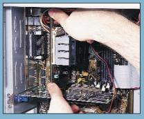
8 Now it's time to insert the slocket, complete with heatsink, into the empty Slot 1 interface on the otherboard. Turn it so that the heatsink is on the same side as the original Pentium II cartridge – this is normally with the heatsink furthest from your external ports. Now line up the slocket carefully inside the retaining clips, and gently but
