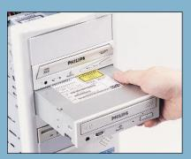
**3** Now physically fit the DVD-ROM drive, by opening the PC case and sliding the drive into a spare 5.25in bay, usually below the existing ROM drive - you will also have to unclip a plastic panel on the front of the case to access the drive once it's fitted. Once slotted into its spare bay, screw it in securely. If there's only room for one 5.25in drive, then you'll need to replace your existing ROM drive with the new DVD model.
