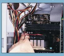
**9** With the slocket in the slot and the retaining clips holding it firmly in place, it's time to connect the power plug for our new CPU cooling fan. This simply goes into the same plug where the old one was disconnected – it'll normally be labelled CPU-FAN on the motherboard. This plug has three pins, so make sure it's connected properly. It'll also only connect one way round.
