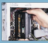
A Now we can remove the entire Pentium II cartridge. This is held in its slot by plastic retaining clips, which vary from system to system. Some should be pulled slightly outwards, while others simply require levers at the top of the clips to be pushed inwards. Either way, they will release the cartridge and allow it to be gently but firmly pulled out of its slot. Place it in an anti-static bag for protection
