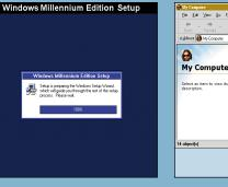
**1 O** Windows will go through its normal installation process. This takes about 30-60 minutes and may ask for some information including the serial numbe (printed on paper inside the CD case), so make sure it's to hand. If Windows tries to start up from the old disk. switch off vour PC and unplug the power cable to the old disk until your new installation is complete. You may prefer to have your old disk unplugged to ensure you don't accidentally repartition or format it in steps 8 and 9.
