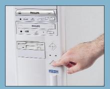
2 You're now ready to switch on your PC. First things first: if nothing appears on the screen, and/or the PC starts beeping furiously, then switch it off and ensure the CPU/Slocket is properly pushed into its slot. If everything's OK, the system will start and briefly identify the new chip. If you're not sure, get a copy of WCPUID from the FTP download section of www.h-oda.com and run it in Windows to identify the chip.
