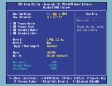
7 Your PC will now need to be told about the disks in its BIOS, so turn it on and press the DEL key to enter the Setup pages. BIOS settings vary, but you should normally start on the first page labelled Standard CMOS Settings, and set both the Primary Master and Slave to AUTO. You may also have to Enable the Primary Master and Slave in the Advanced CMOS Settings. Finally, choose to Exit **Saving Changes.**
