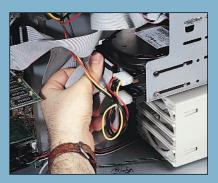
The flat wide 'ribbon' data cable Should be unplugged from the old hard disk and inserted into the new one This cable will have another connector halfway along it, and this should be plugged into the old disk. If your cable doesn't have plugs for two drives, then you can buy a new one for about £10. Finally, connect a spare power plug to the new disk. This will have four coloured wires going into it.
