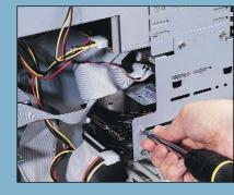
The next step is to open the case and nount the new hard disk. Most larger cases have space to accommodate at least one extra hard disk, so it should be easy to slide the new disk into a spare bay and screw it in securely at the sides. If your case doesn't have room, follow the rest of the steps and, once completed, remove the old disk and slot in the new one in its place.
