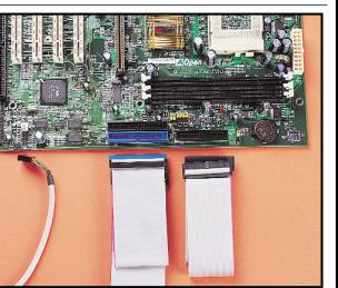
Make sure you have all the components you require to build a completely operational PC. New memory or a CPU may be top of your list, but they'll be useless if you're missing an essential system cable. Most motherboards will come with an EIDE cable to connect to a hard disk, and suitable retention clips if it's a slotted CPU model, but ensure they're compatible with your components.
