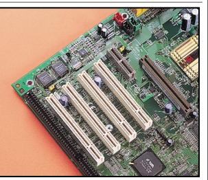
Almost all motherboards will have the same plugs as your old one, letting you recycle your input devices – although ancient AT keyboards may not work. The PCI standard hasn't changed, so any existing cards should also work. There are unlikely to be any ISA slots, and PCI graphics cards are best upgraded to AGP. UltraDMA33 drives will work on newer UltraDMA66 and 100 interfaces.
