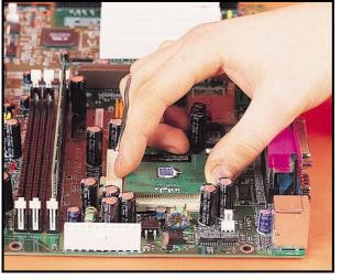
To fit a slotted CPU, insert the vertical retention clips into the 2 motherboard, then slide the CPU cartridge into its slot. To fit a socketed CPU, lift the lever on the side of the socket and drop in the processor, align the pins then push down. Clip on the heatsink, and connect the fan's power cable. To fit memory, pull back levers at each end of the slot, push the card in, then lock levers into card's notches.
