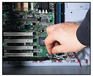
Reattach the right-hand case panel, insert all the cables, 4 including the power connector, the flat-drive ribbon cables and the wires for the front-panel lights and buttons. Refer to the manual to connect them correctly. Ribbon cables have one coloured wire, which should be aligned with the side of the socket with a number 1 next to it. Finally insert the cards and screw them in securely.
