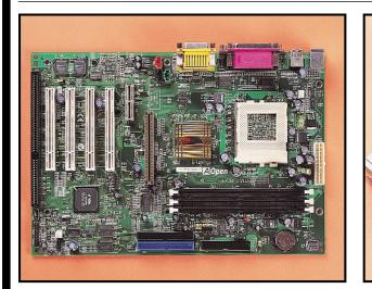
The key to upgrading is deciding which existing components can be recycled. First, ensure a new motherboard will actually fit in your existing case. Virtually all new motherboards use the ATX form factor, requiring an ATX case and power supply. If your case is pre-ATX, other existing components could also be dated, and you'd be better off buying a new PC instead.
