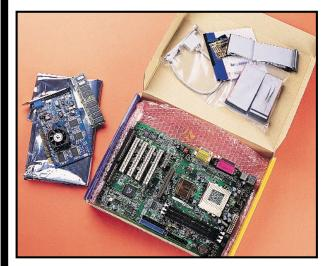
Before fitting your new motherboard, familiarise yourself with it and all the components you're going to insert. Ensure you've got plenty of room to work with, and safe places to store components while they're outside of the PC - the silver anti-static bags that new cards and motherboards are supplied in are ideal. Make sure you're grounded, as static electricity can instantly destroy PC components.
