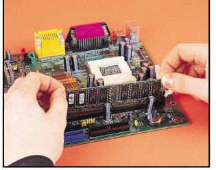
Now that you're fully prepared, it's time to fit the new 1 motherboard in your case and reconnect all the cables. As with the removal stage, you may find it easier to fit the CPU and memory onto the board before screwing it into the case - this is the order in which we'll do it, but there's nothing stopping you first screwing the board in the case then reaching inside to fit the required components.
