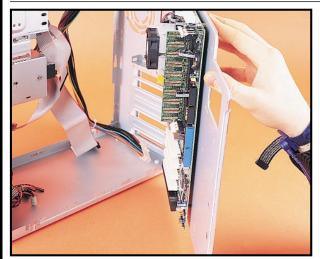
Now you must fit the board in the case, although you can do 8 Now you must ne the board in an either lower the this before step two if desired. You can either lower the motherboard into the case, or remove the case's right-hand panel for direct access. The motherboard itself is held in by several screws around its edge and a couple in the middle - these align it with the holes in the case and prevent it from lifting when cards are pulled out.
