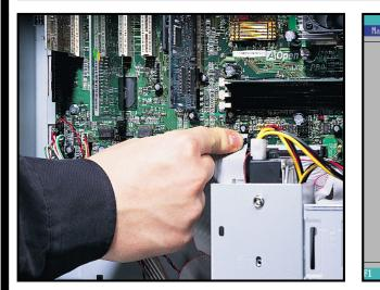
With all components, cards and cables correctly inserted and verified: connect all the external cables and switch the power on. If nothing happens, switch off and check the cables are the right way round. Ensure the CPU, memory and cards are fully inserted - a gap will stop it powering up. If your system beeps, count the number and cross-reference it with the troubleshooting guide in the manual.
