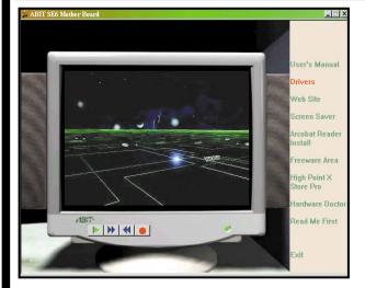
Now start up your operating system. A motherboard requires 3 the right drivers to make it work. Windows will detect new devices and install the software for them. It's also essential to install the drivers that came with the motherboard for best performance. Owners of motherboards with VIA chipsets should check VIA's website w.via.com.tw) and download the latest 4-in-1 driver.
