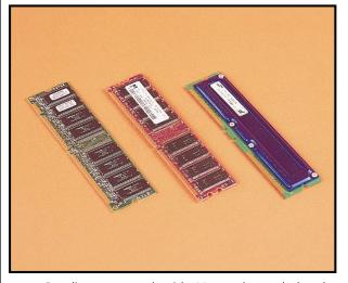
Recycling memory can be tricky. Most modern motherboard 3 and CPU combinations require SDRAM DIMMs running at a specific speed, and unless yours match the specification, you can't re-use them. Also, DDR SDRAM and RDRAM motherboards require their own type of memory that's not compatible with conventional SDRAM. If you want new memory, go for a faster DDR motherboard.
