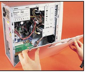
Every PC case opens differently, but your goal is to remove the left-hand side panel with the PC facing you. This could involve removing several screws and/or unlocking a latch. Once opened, you should lay the PC on its closed side, providing easy access to the insides. A well-lit work surface with plenty of static-free room to lay out components is an advantage - your carpet is not a good surface.
