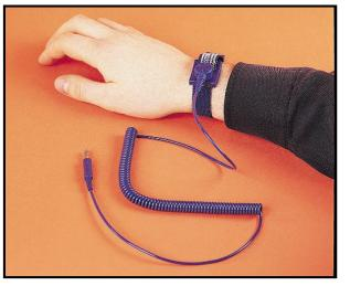
Once you've decided what to recycle, open your PC case and sensitive PC components, so ensure you're grounded. Some people touch the metal casing of the internal power supply to do this, more cautious upgraders should invest in an anti-static wrist strap and avoid nylon clothing. Also remove all plugs from the back of your PC.
