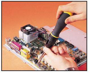
Unscrew the motherboard. Take out memory cards by pulling 4 back the levers at each end to release them. The entire cartridge of a slotted CPU is removed by pulling outwards on the tall clips on either side, and lifting. A socketed CPU must have its heatsink unclipped before pulling up the lever on the side, allowing the CPU to be lifted out. Remember to unplug the CPU fan's power cable.
