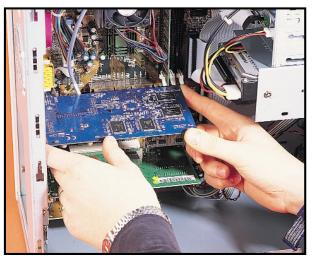
Once inside the PC, remove all cables and cards connected to 3 the motherboard. Start by unscrewing the card's retainers and firmly pulling them out one by one. Next disconnect all the cables from the motherboard, including the flat ribbon drive cables, the multicoloured power connection, and the thin wires that make the lights and buttons on your PC's front panel work.
