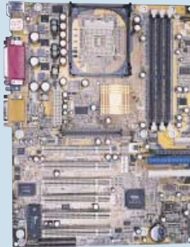
Azza's P4X2-AV motherboard is based on a chipset that supports DDR SDRAM
