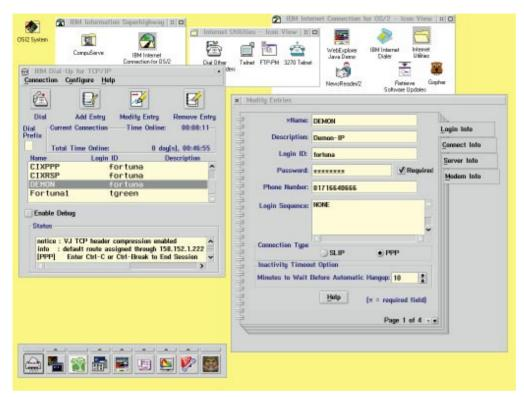
To set up the DOIP dialler, choose to add an entry and fill in the details on all four pages. Select PPP for Connection Type on page one; enter Login ID (your CIX-IP login name) and Password on page one of the dialler notebook. Enter the IP address of your host for CIX or Demon, and the nameserver IP address on page two. Fill in the modem details on page four.
