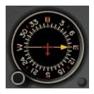
The Automatic Direction Finder (ADF) is used to track NDBs. The Non-Directional Beacon is a form of navigation that allows you to fly between two locations using ground-based transmitters and aircraft receivers.
