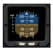
The electronic attitude indicator on the CitationJet serves four functions: artificial horizon; angle of attack (AOA) indicator; Course Deviation Indicator (CDI) during VOR tracking and ILS approaches; and glide slope indicator during ILS approaches.
