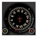
The heading indicator, or directional gyro, operates on an internal gyroscope that provides accurate heading information *once it is set to the correct heading using the magnetic compass.* This should be done by the pilot prior to taxiing. Click (and hold) to the left or right of the knob at the lower left edge of the instrument to rotate the indicator clockwise and counterclockwise. The airplane's heading then appears at the top of the instrument.
