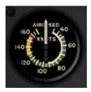
The airspeed indicator uses the ram air from the pitot tube, compares it with the static air pressure and converts it to Indicated Airspeed which is displayed on your airspeed indicator. Modern airspeed indicators show knots on the outer scale and mph on the inner scale. There are three definitions of airspeed:
