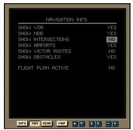
The selections are the same as when a flight plan is loaded, however FLIGHT PLAN ACTIVE will be automatically toggled to NO. Also, you will not see the subsequent menus that show flight plan leg information.
