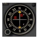
The NAV instrument is used in VOR/DME navigation primarily as an indicator of the airplane's position relative to a referenced radial on a VOR. It is also used to track localizers during ILS approaches.
