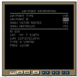
To toggle between the INFO map and the INFO menu, click the MAP button. On the menu, the selections, as they are referred to here, are listed on the left. The options are listed on the right. To toggle up and down between options, click the up and down arrow buttons on the GPS Receiver. To toggle between options for each selection, click the left and right arrow buttons on the GPS Receiver. The INFO menu has three selections:
