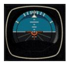
The **attitude indicator** is also called the artificial horizon. It shows the relationship of the nose and wings to the horizontal plane. All movements of the flight controls, such as changing pitch or bank, are done by direct reference to this instrument.
