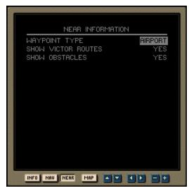
To toggle between the NEAR map and the NEAR menu, click the MAP button. On the menu, the selections, as they are referred to here, are listed on the left. The options are listed on the right. To toggle up and down between options, click the up and down arrow buttons on the GPS Receiver. To toggle between options for each selection, click the left and right arrow buttons on the GPS Receiver. The NEAR menu has three selections:
