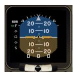
The electronic attitude indicator on the Super King Air serves four functions: artificial horizon; angle of attack (AOA) indicator; Course Deviation Indicator (CDI) during VOR tracking and ILS approaches; and glide slope indicator during ILS approaches.
