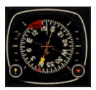
The Horizontal Situation Indicator (HSI) is a combined heading indicator and VOR display. It comprises a course index (yellow arrow), a heading bug (red pointer), a Course Deviation Indicator (yellow bar), a glide slope deviation indicator (white line scale on sides of compass rose), and a TO-FROM indicator (small white triangle near center of compass rose). The red HDG flag is a power off indicator. The red NAV flag indicates that no navaid is tuned in for the VOR.
