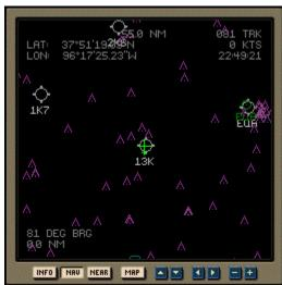
When no flight plan is loaded, the NAV map only displays the information that is toggled on in the NAV menu.
