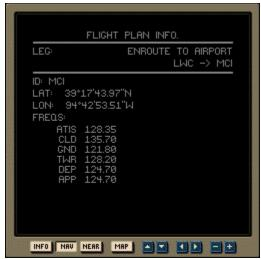
After your selections are made in the NAV menu, click the MAP button once to see a subsequent menu that contains information about the first leg of the flight plan. When this menu is displayed, click the left or right arrow buttons to scroll through each leg of the flight plan. The departure and destination waypoints of the leg appear in the upper right of the screen.
