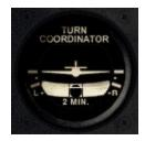
The **turn coordinator** consists of the bank indicator (the miniature airplane) and the slip-skid indicator (the floating ball). The bank indicator shows two hash marks that indicate standard left and right turns. In instrument flight, all turns are made at a rate of 3° per second. At this standard rate, a complete 360° turn is made in two minutes. Smaller turns (5-10° heading changes) require a less-than-standard rate turn.
