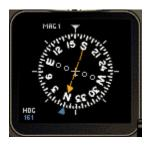
The Electronic Horizontal Situation Indicator (EHSI) is a combined heading indicator and VOR display. It comprises a course index (orange arrow), a heading bug (blue pointer), a Course Deviation Indicator (orange bar sometimes aligned with course index), a glide slope deviation indicator (scale to the right of compass rose), and a TO-FROM indicator (small white triangle near center of compass rose).
