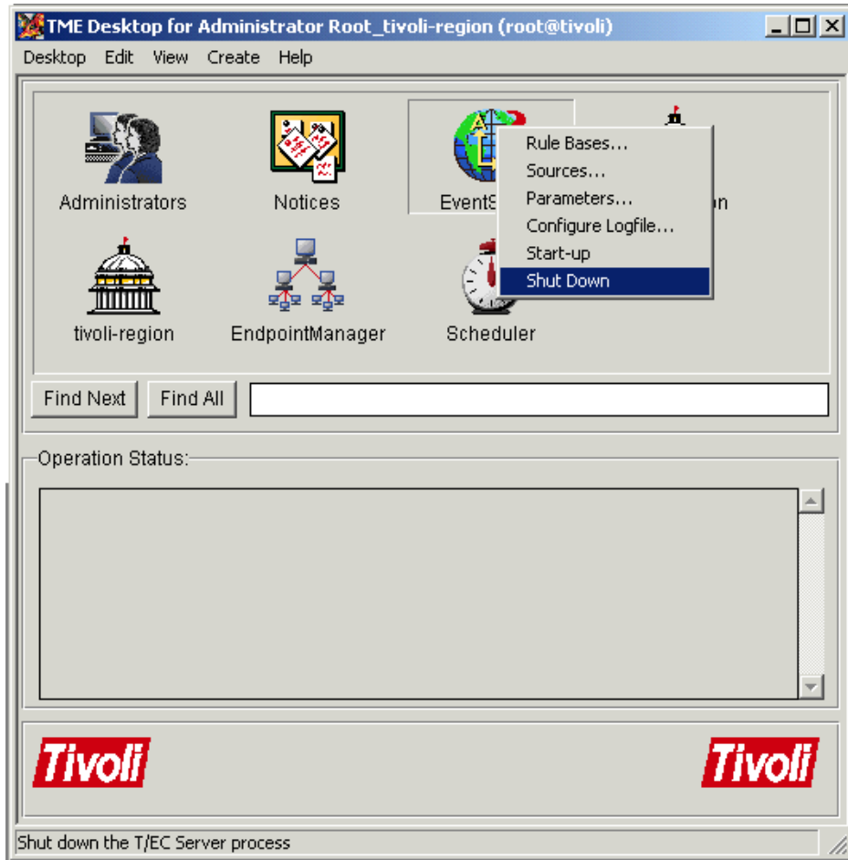
Figure 36. Shut down the Event Server
