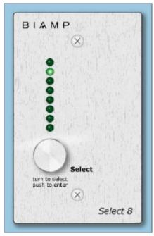
The Select 8 is an external control device, which allows initiation of eight selectable NEXIA actions. Actions can be individual or grouped functions within NEXIA. This includes recalling presets, ducking, combining, etc.
