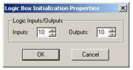
The Logic Box is an external control device, which provides twenty logic input/output connections. When a Logic Box is placed, an Initialization Properties dialog box appears for assigning the quantities of logic inputs/outputs (20 total). Logic inputs allow external switches to initiate NEXIA actions. Actions can be individual or grouped functions within NEXIA. This includes recalling presets, ducking, combining, etc. Logic outputs can be used to control additional equipment, external to NEXIA.
