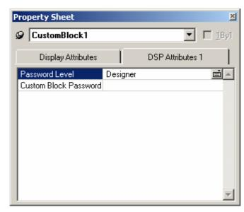
Control settings also remain part of any Custom Block which has been copied into the Processing Library. These control settings may again be addressed once the Custom Block is placed into a new NEX design file. However, to prevent tampering with control settings, password protection may be added to a Custom Block via the Property Sheet. This option is available only while working in the Custom Block NEX file.
