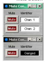
**Mute** turns on/off the channel. **Identifier** provides a custom label, when the dialog box is minimized (see below).
