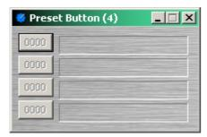
Right-clicking over a button provides a list of available Presets which can be assigned to that button. The Preset Number will appear on the button, and the Preset Name will appear to the right. Preset Numbers can be replaced with the word 'Recall' (see General Options). Control Dialog Boxes for Preset Button components can be minimized to create user control surfaces (see Customizing Component Objects).
