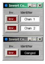
**Invert** reverses the polarity of the audio signal (180°). **Identifier** provides a custom label, when the dialog box is minimized (see below).
