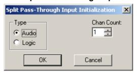
Split Pass-Through blocks allow associated input and output wiring nodes to be placed in separate locations, with an implicit or 'wireless' connection being maintained between them.
