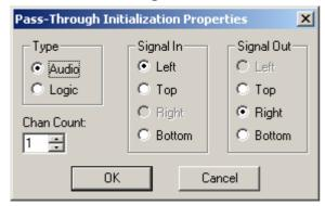
Pass-Through blocks allow wiring nodes to be strategically placed, so audio or control (logic) signals can be routed in different directions.
