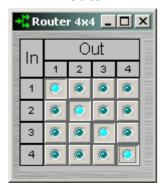
Routers allow each input to be assigned to multiple outputs via **In / Out**. However, each output allows only one input assigned at a time. Therefore, Routers behave like a series of individual distribution amplifiers. For increased input/output assignment capability, see Mixers.
