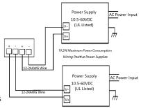
Power should be disconnected from the power supply before connecting it to the switch. Otherwise, your screwdriver blade can inadvertently short your terminal connections to the grounded enclosure.
