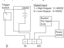
external DC type signal input and can be configured to send alert message through Ethernet when the signal is changed.
