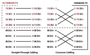
Connect one side of an Ethernet cable into any switch port and connect the other side to your attached device. The LINK/ACT LED is lit when the cable is correctly connected. Always make sure that the cables between the switches and attached devices (for example, switch, hub, or workstation) are less than 100 meters (328 feet).
