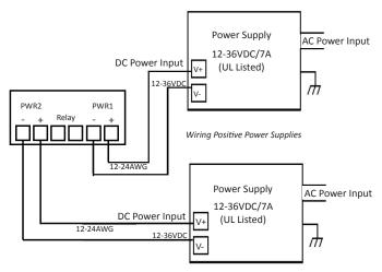
Power should be disconnected from the power supply before connecting it to the switch. Otherwise, your screwdriver blade can inadvertently short your terminal connections to the grounded enclosure.
