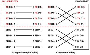
Always make sure that the cables between the switches and attached devices (for example, switch, hub, or workstation) are less than 100 meters (328 feet). You should use Category 5 cable or higher.
