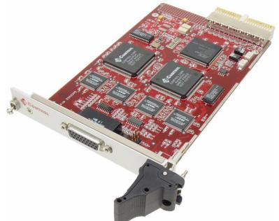
The RocketPort CompactPCI uses Application Specific Integrated Circuits (ASICs) technology to replace most hardware components, including the processor and the serial controller. You can install up to four RocketPort CompactPCI boards in one PC, for a total of 64 additional serial ports.
