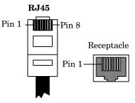
Building RJ45 Loopback Plugs Loopback plugs are used with the diagnostics to test serial ports. This RJ45 loopback is used with the Rack Mount interfaces.
