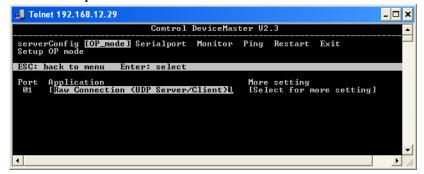
Press the **Enter** key to activate the short-cut menu that displays the four **Operating Mode** options: **Host Based**, **Pair Connection (Master)**, **Pair Connection (Slave)**, and **Raw Connection**. Use the up and down **arrow keys** to select the desired setting, and then press the **Enter** key. The new setting, enclosed in square brackets will appear to the right of the **Operating Mode** category.
