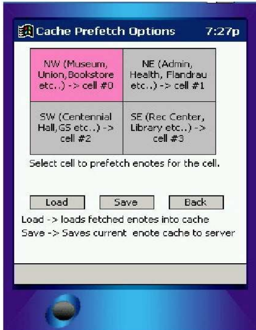
Figure 3: The pink region is where the user is currently located. By clicking on any of the (other) cells he can prefetch the data for that cell.
