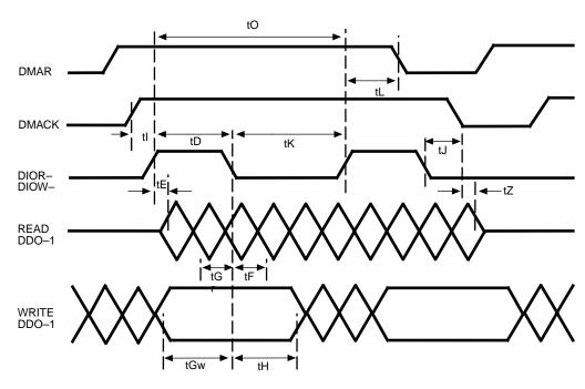
Detailed view of Multiword DMA timing diagram
