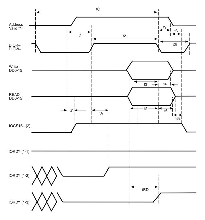
Detailed view of PIO Timing Diagram
