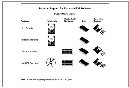
Fast ATA and Fast AT-2 represent only the fast data transfer rates for ATA hard drives (support for PIO Mode 3 or 4 and DMA Mode 1 or 2). Fast ATA and Fast ATA-2 data transfer rates can easily be achieved when the system BIOS and hard drive support the PIO and DMA protocols. Fast ATA BIOS have been included in popular computer systems since 1993.
