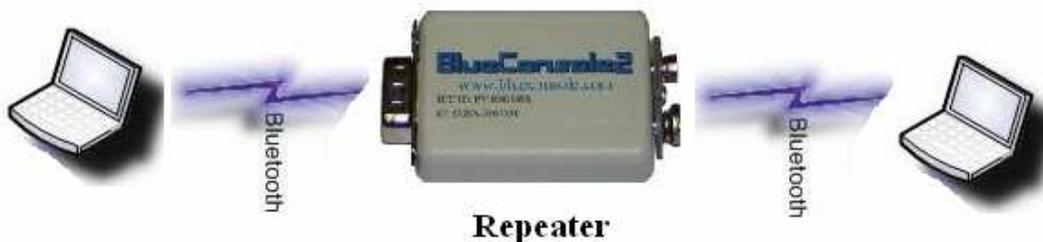
**Case 2:** Extend the Bluetooth distance from a PC/Mac/PDA device to a native RS232 device equipped with a BlueConsole adapter or integrated Bluetooth.
