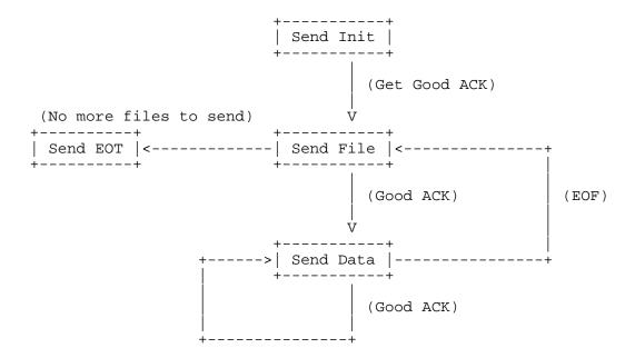
Base-level KERMIT provides that during any particular transaction, the sender is the "master" and the receiver is the "slave". These roles may be reversed in the next transaction; any KERMIT implementation is capable of acting as either master or slave. In addition, mainframe implementations may also be put in a kind of permanent slave, or "server", mode in which all commands come in command packets from the master, or "user" KERMIT.
