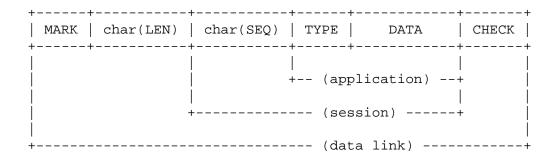
where all fields consist of ASCII characters, and the *char* function converts a number in the range  $0-94_{10}$  to a printable ASCII character by adding  $32_{10}$ .
