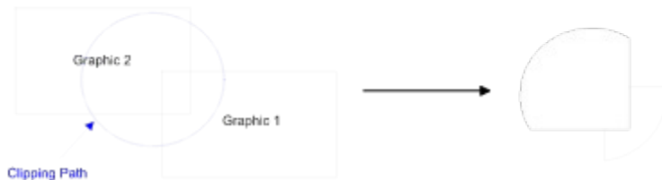
The results of multiple closed graphic primitives used on a clipping path.
