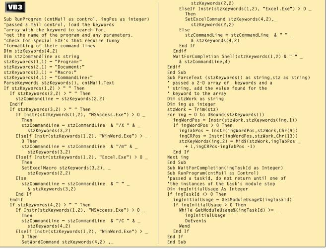
LISTING 2 Looking for Keywords. The ParseText routine provides a standard way for each message-type routine to find its keywords. With VB4's improved variants, you can implement this as a function. RunProgram is the workhorse routine in MailHandler and shows how the ParseText routine is used. WaitForCompletion uses a Windows API call to pause MailHandler until the program completes.
