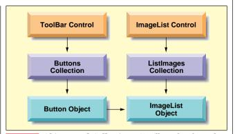
FIGURE 1 **Objects and Collections.** You'll need to know how these objects relate to each other to develop a working toolbar. The toolbar buttons are a collection of Button objects with their own properties and methods. And to make it a bit more complex, the images on the button faces are contained with the ListImages collection of an ImageList control.
