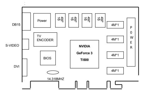
NOTE 1: TV output connector and encoder are reserved for optional NOTE 2: DVI connector and LCD encoder are reserved for optional
