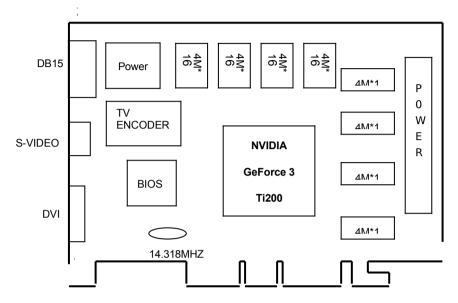
NOTE 1: TV output connector and encoder are reserved for optional NOTE 2: DVI connector and LCD encoder are reserved for optional
