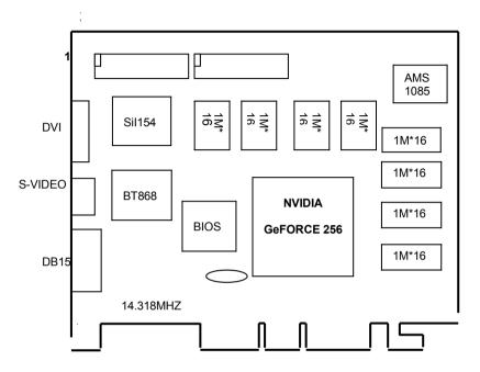
NOTE 1: TV output connector and encoder are reserved for optional NOTE 2: DVI connector and LCD encoder are reserved for optional
