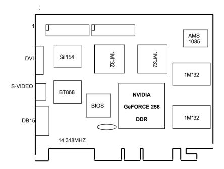
NOTE 1: TV output connector and encoder are reserved for optional NOTE 2: DVI connector and LCD encoder are reserved for optional
