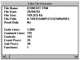
The Code Lines total is the actual coding lines in the project - it does not include comments, blank lines or any of the control definitions.
