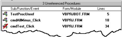
The <u>Lines column</u> notes how many coding lines appear in that procedure. The percent bar will be displayed whilst the report is created.
