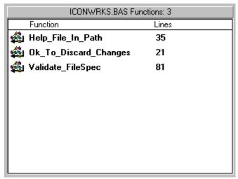
The <u>Lines column</u> notes how many coding lines appear in that procedure.
