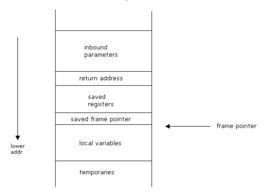
The figure above illustrates the stack frame used by LCC. Here's a timeline of the implementation of function calls:
