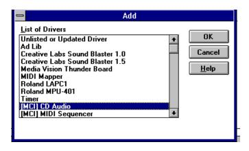
(4)Select [MCI] CD Audio and click OK button add this driver to your Drivers. Windows may ask you to insert a Windows installation disk to load this driver. When [MCI]CD Audio driver has been loaded and your CD-ROM driver has been installed properly, a pop-up window will display a message which will tell you a CD-ROM driver has been detected.
