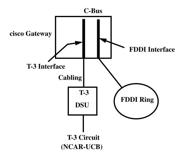
Figure 2 Hardware Configuration (Identical at Both Ends)
