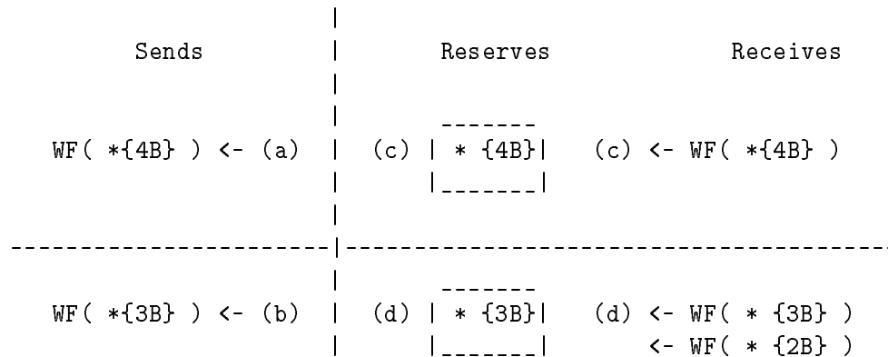
Figure 8: WF Reservation Example – Partial Routing
