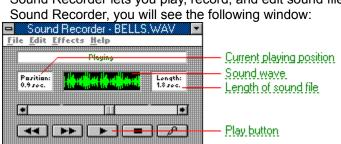
To play a file, click the Play button. As the sound plays, the Wave box graphically displays the sound as if it were being shown on an oscilloscope.
