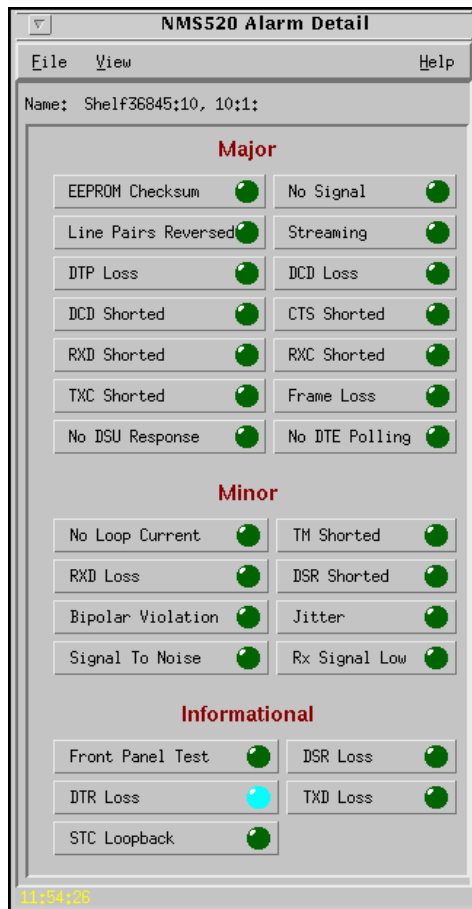
Figure 6-3 Alarm Detail Window
