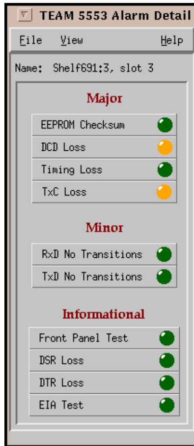
Figure 2-2 Alarm Detail Window
