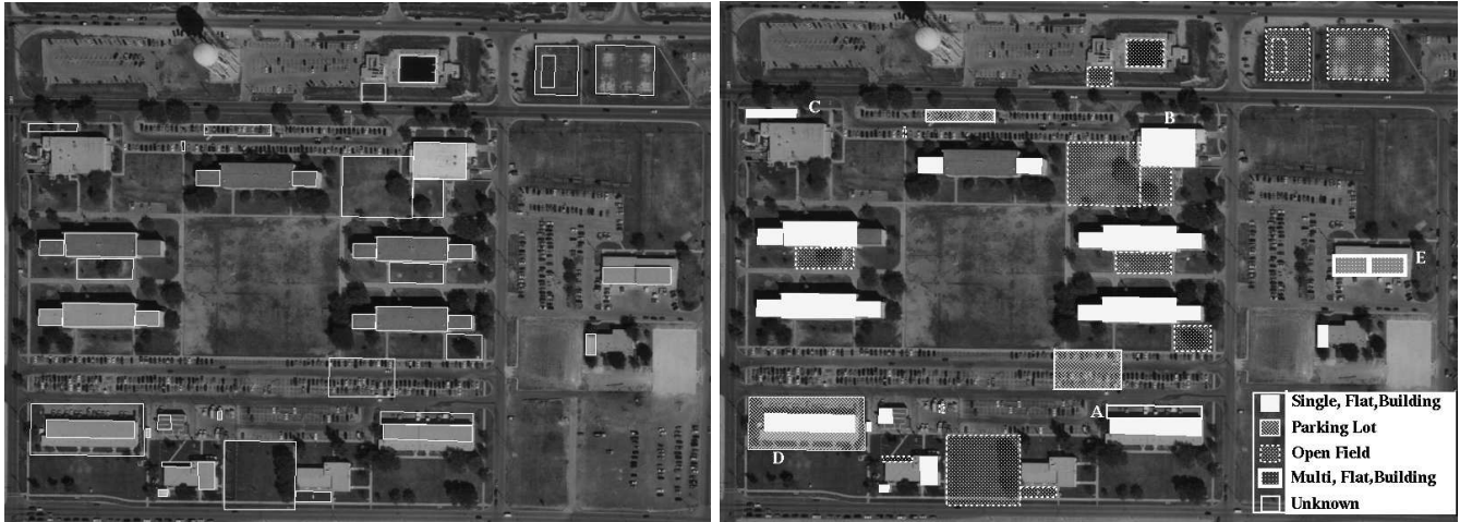
Figure 10: (a) Regions produced by the Ascender system used for classification. 22 polygons correspond to building rooftops. (b) Classification results. Four regions were misclassified and in two other regions the system was not able to decide on the classification. Letters referred to in the text.
